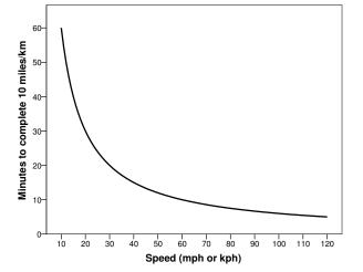
Figure 2: The "Paceometer"—A speedometer showing values of pace (minutes per 10 miles) at selected levels of speed (mph).
